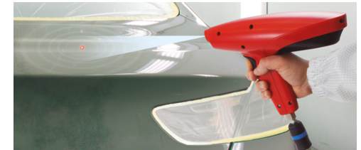
4. Pull the trigger. The laser indicates the area that is being decontaminated and ionizing.
