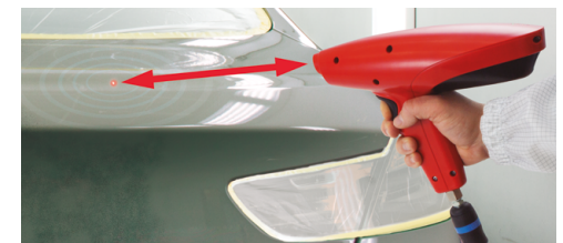
5. Application is the same as painting, without changing the distance, speed or pressure.
